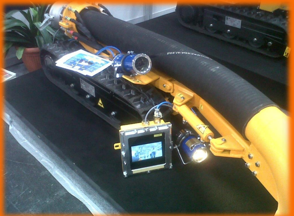
Figure 1: Camera & Led ATEX zone 0 and Monitor ATEX zone 1 combined with Lombrico R
