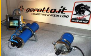
Figure 2: ATEX zone 0 Camera & Led and Monitor ATEX zone 1
