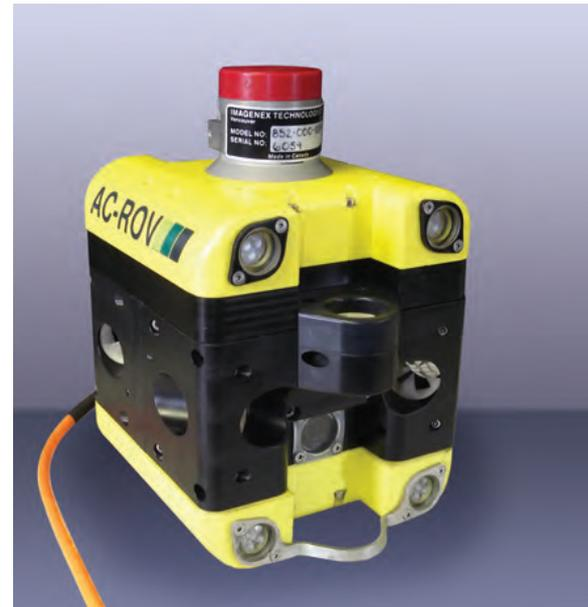
The model 852 Digital Imaging Sonar has been customised for use with the **AC-ROV 100** to offer the world's smallest scanning sonar ROV package.
